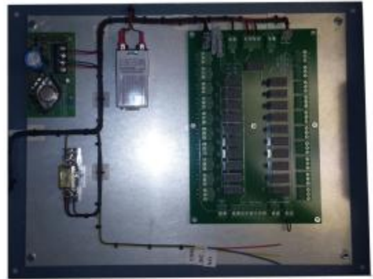
The Main Control Board and DC Power Supply
